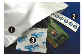
① Moisture Barrier Bag ② Humidity Indicator Card (HIC) ③ Desiccant
